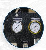
Liquid Filled Panel Mounted Concentrate Pressure Gauge
